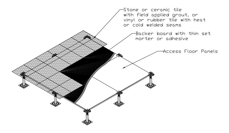
Suitable for use with virtually any conventional floor finish. In addition, provides a waterproof solution when used with the appropriate floor finish.
