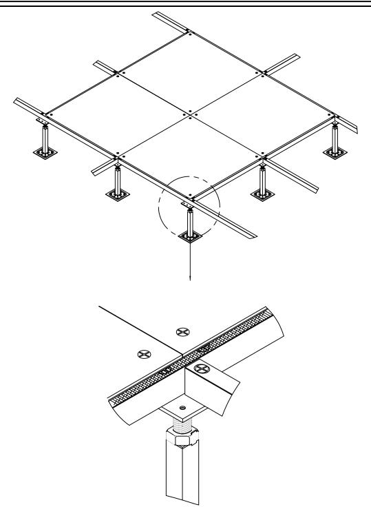
Field applied gasket on stringer with monolithic vinyl or rubber tile. Install with Combo Screws. (Water resistant, not waterproof) McMaster Carr #93745K53 - 3/4" wide gray, firm
