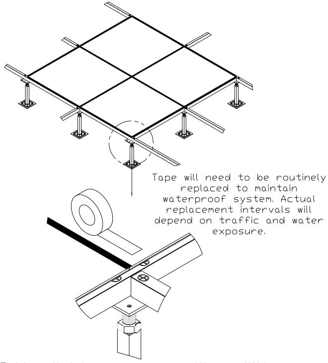
Field applied tape over seams with monolithic or top set trim vinyl or rubber tile.
